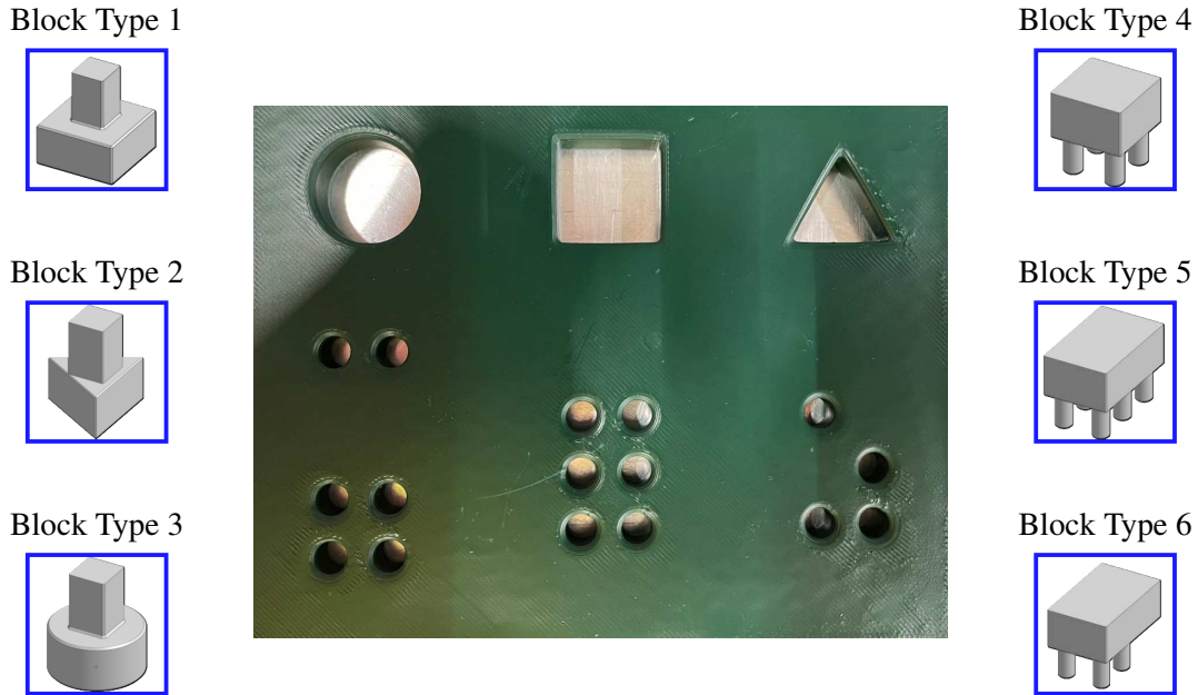
Figure 4.4: The presentation of the test bed with 3D-printed blocks. The blocks differ in shape and size. In this test bed, the clearance of insertion holes is 2 mm
